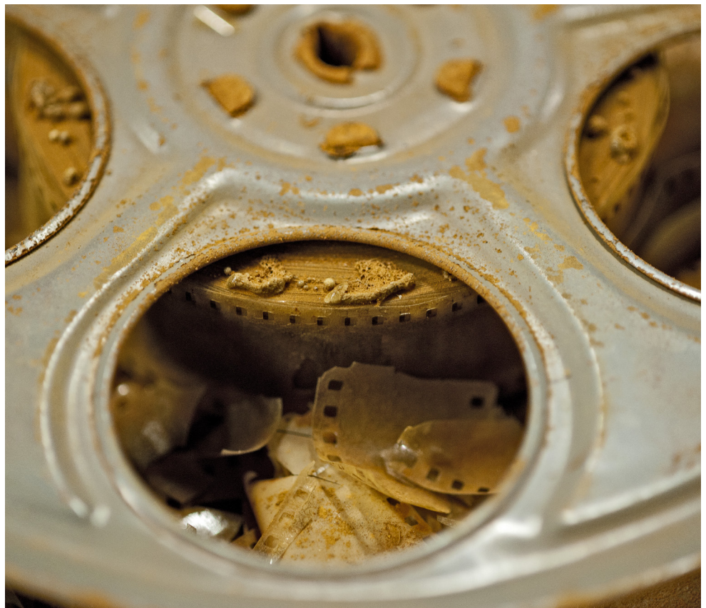
In addition to the ravages of time, mid-20th century film reels used for capturing events from atmospheric nuclear tests were subjected to radiation damage. Film crews attempted to protect cameras from radiation exposure with lead and concrete shielding and by positioning them at lower risk distances from ground zero. This reel from the first nuclear weapons test (in New Mexico in 1945) is beyond repair. (Photo by Lee Baker.)
