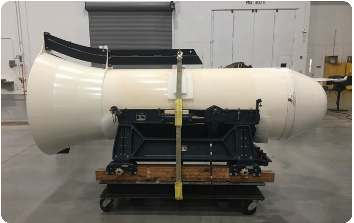
Above - AVCO Mark IV Re-entry Vehicle, used in the Atlas 8F and Bluegill Triple Prime tests
